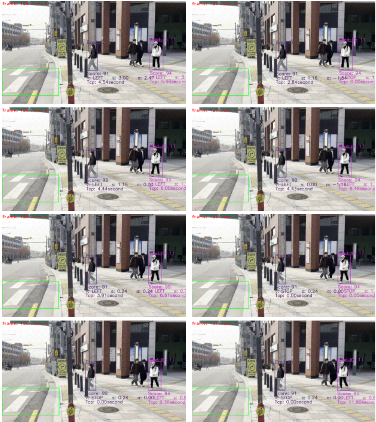
Figure 12. An example of detecting multiple pedestrians approaching a crosswalk (direction: v, speed: s, acceleration: a, time remaining until arrival at crosswalk: Tcp, status: crossing)
