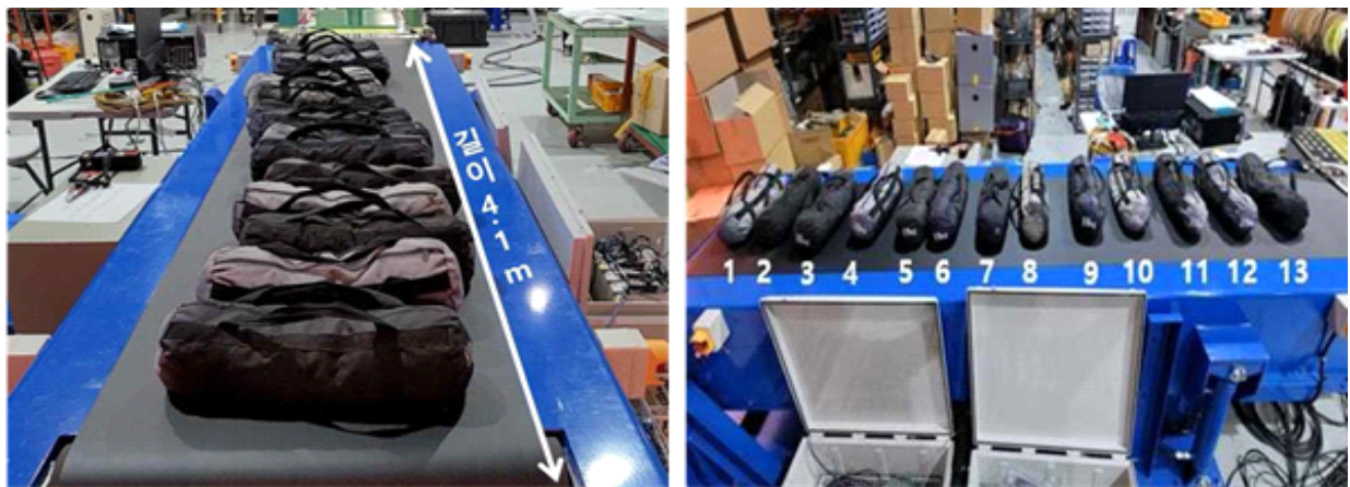
Figure 9. Conveyor carrying load test (Sample)
