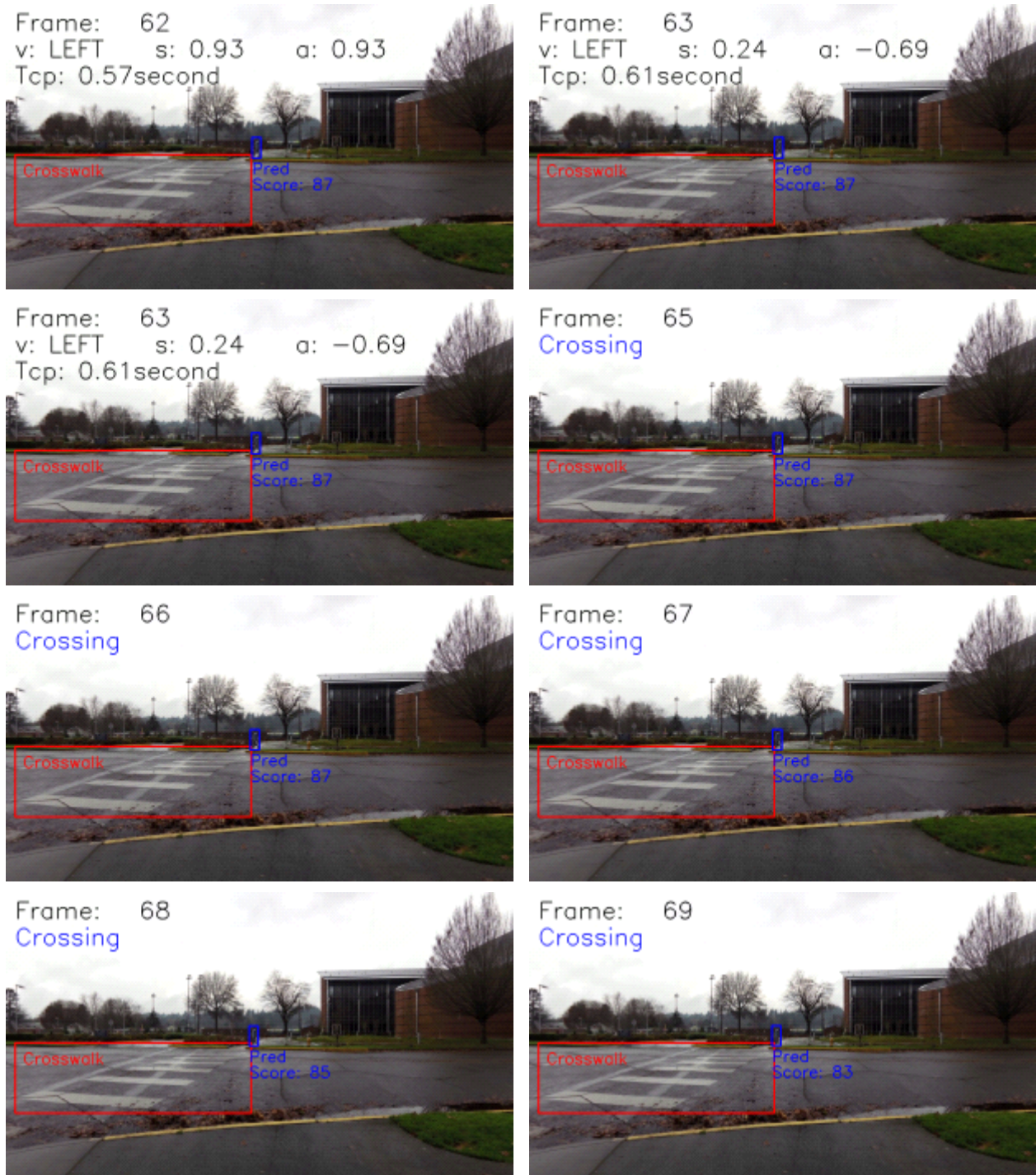
Figure 9. Examples of tracking a pedestrian at crosswalks and estimating the remaining time through eight sequential frames(62-69) (direction: v, speed: s, acceleration: a, remaining time until arrival at crosswalk: Tcp, status: crossing)
