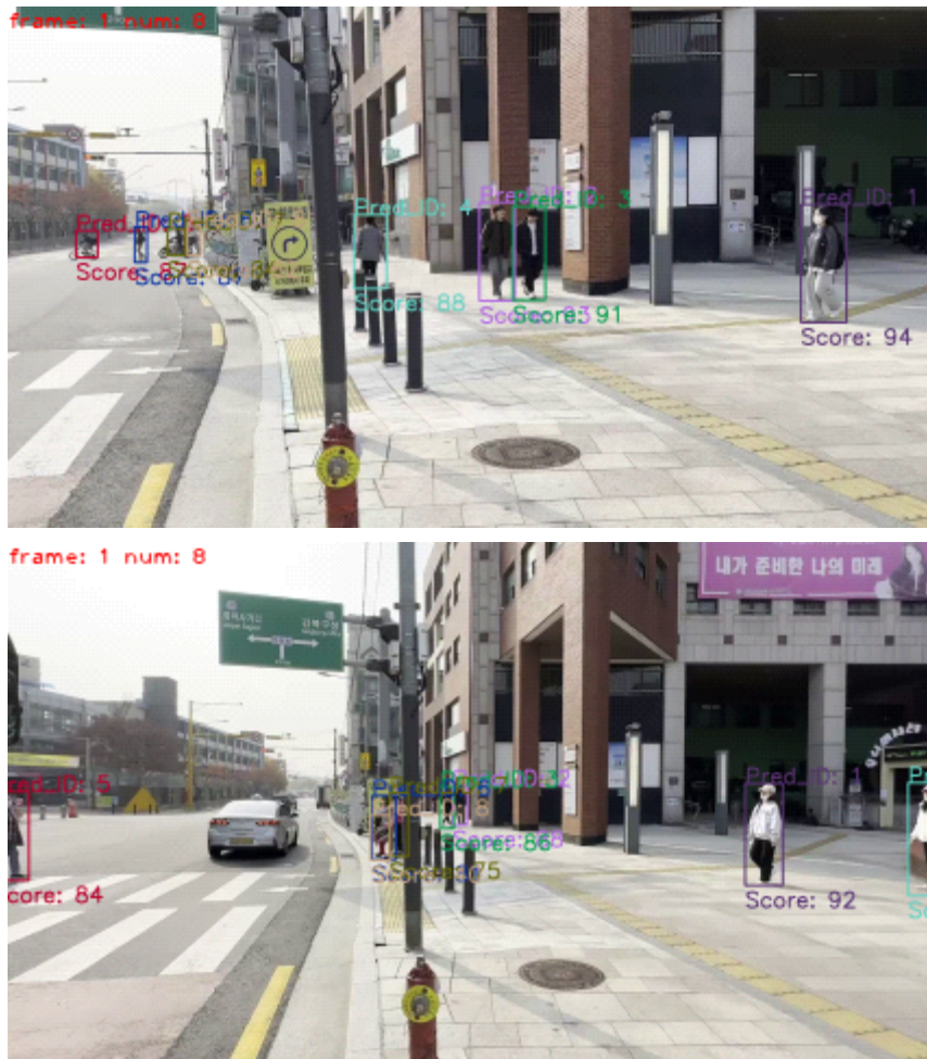
Figure 10. Example of detecting multiple pedestrians around crosswalks
