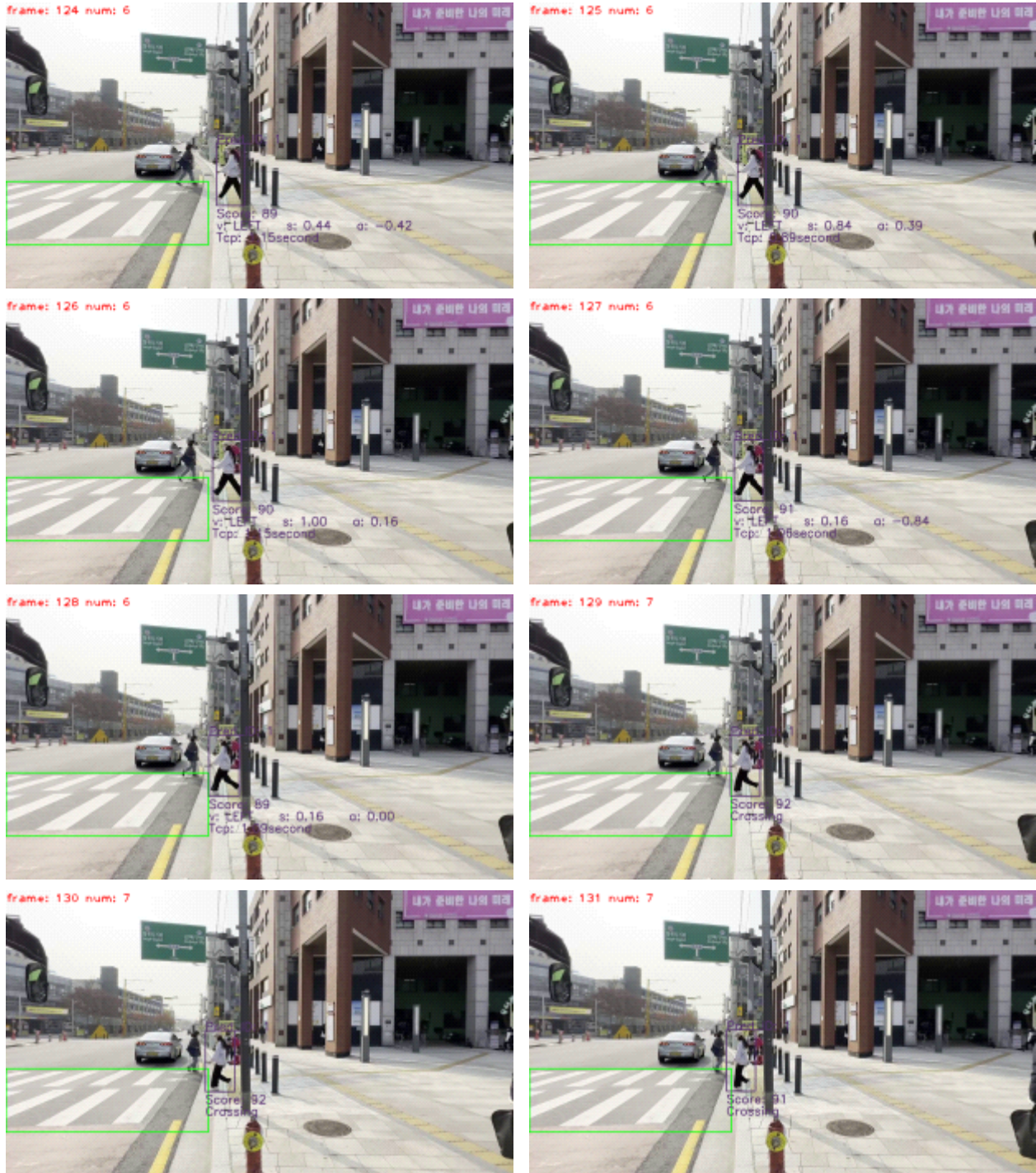
Figure 11. An example of detecting the ID#1 pedestrian approaching the crosswalk (direction: v, speed: s, acceleration: a, time remaining until arrival at crosswalk: Tcp, status: crossing)
